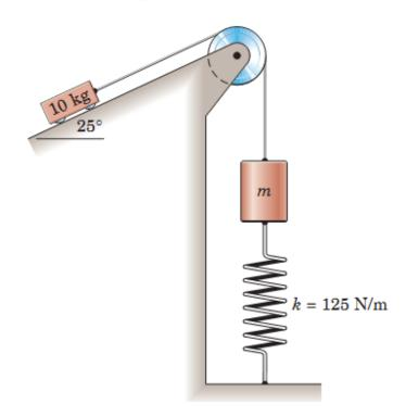
3/107 Let s be the slant distance down the incline traveled by the 10-kg cart.
