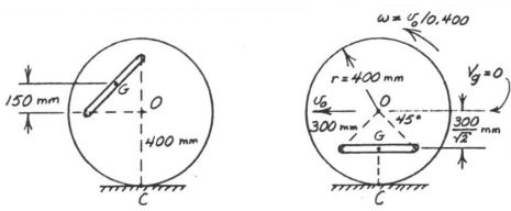
$$V_{G} = \frac{\overline{CG}}{r} V_{O}, I_{G} = \frac{1}{12} 9(0.300 \sqrt{2})^{2} = 0.135 \text{ kg·m}^{2}$$
